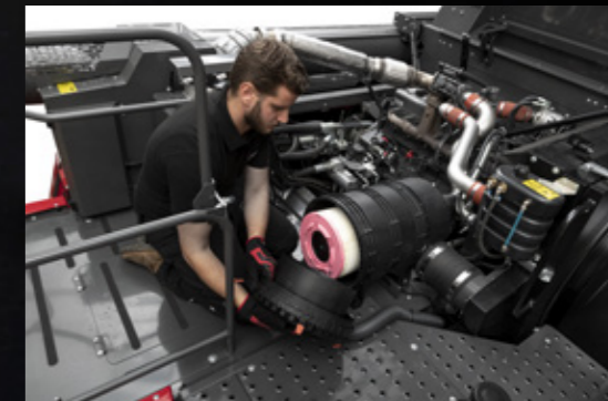
Checking and cleaning the air filter
